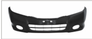
BUMPER FRONT WITH FOG LAMP HOLE
